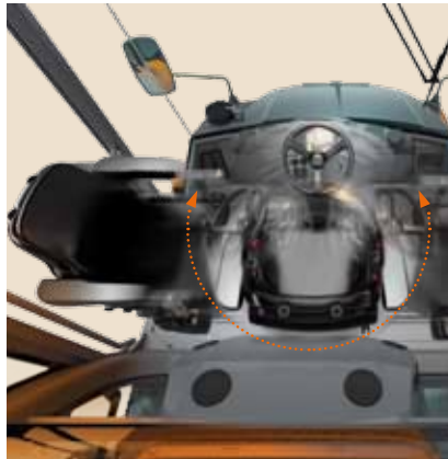
The operator's seat can be rotated 90° to the left or right by a single hand movement.
