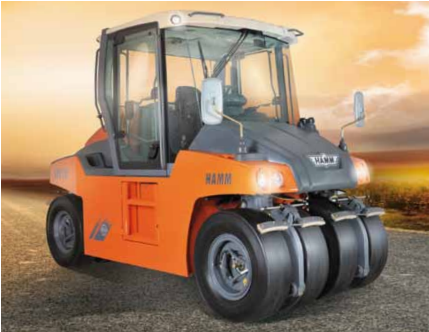
The operator's seat can be rotated 90° to the left or right by a single hand movement.
