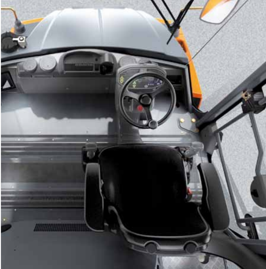
The operator's seat can be shifted to the outer edges of the platform – providing an optimal view of the wheels.
