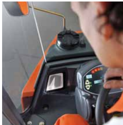
View from the cab: the inner front tire edge as seen through the viewing channel.
