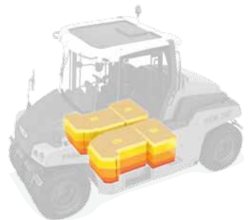
The ballast spaces can be loaded with pieces of varying thicknesses and materials. Thus, machine weight can be adjusted quickly and easily.
