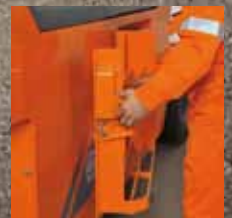
... and relock the steps on the outer frame. Done!
