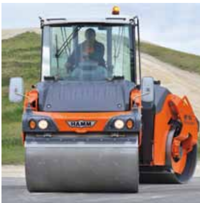
Optimal weight distribution even on sharp turns due to articulated steering.
