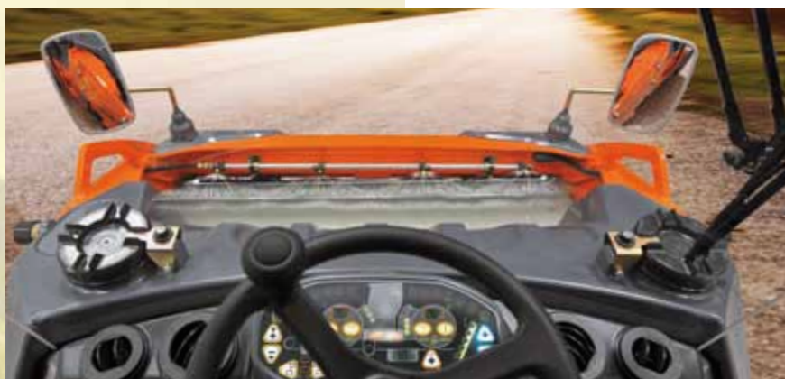
Large rear-facing mirrors for all-round visibility from the XXL panoramic cab.
