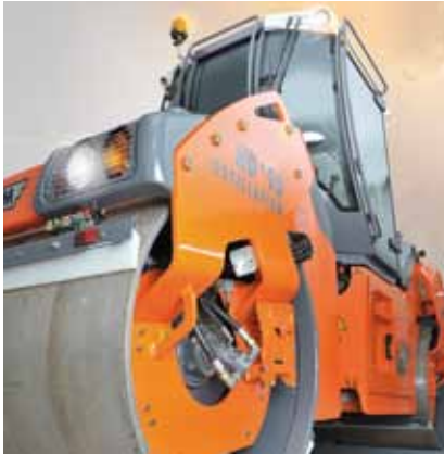
Unrestricted view of the edges of the drum from the operator's platform.
