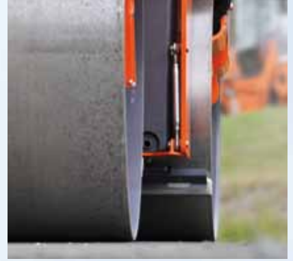
Trouble-free edge pressing thanks to a crab steering mode of up to 6.7" (170 mm).
