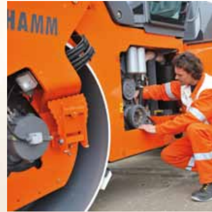
Easy access for rapid servicing: the service and maintenance points are concentrated on the right-hand side of the engine.
