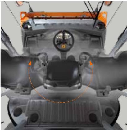
The driver's seat is adjustable and can be rotated 90° in either direction.
