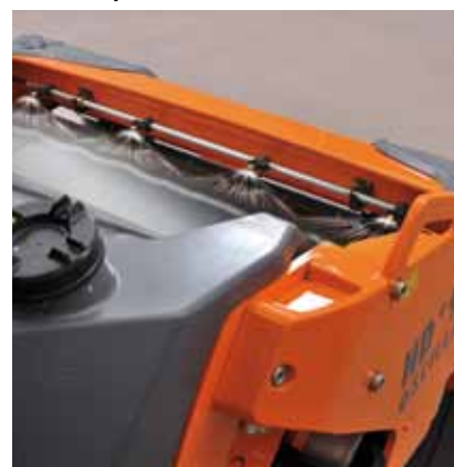
The panoramic cab and the open upper-frame design allow the spray system to be kept in sight at all times.
