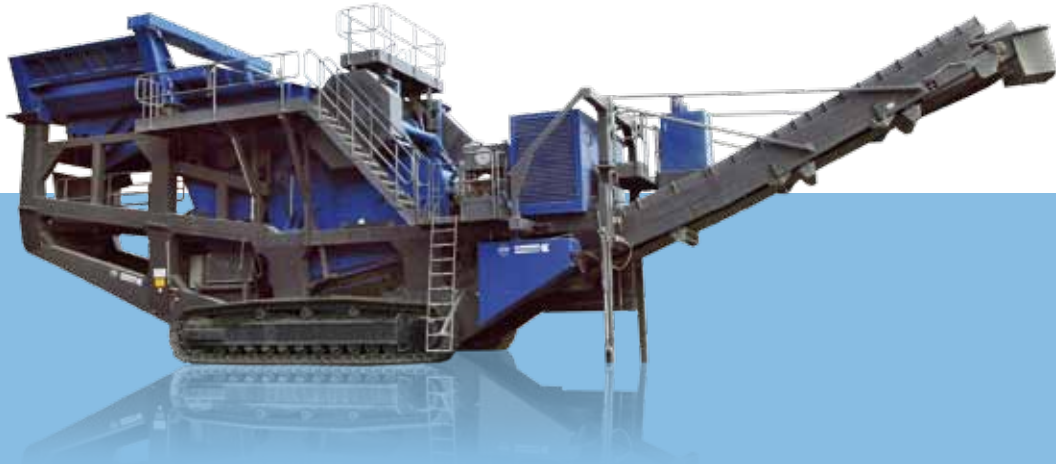
Side view MC 140 Z operating position
