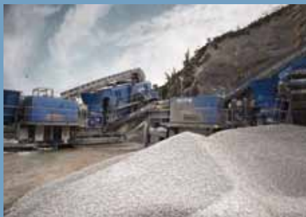
Two mobile cone crushers one after the other from the MOBICONE MCO 13 S.
