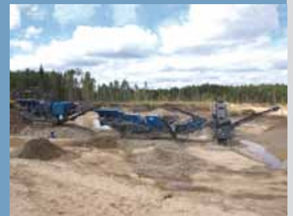
Plant combination consisting of a jaw crusher (MC 120 Z), an impact crusher (MR 130 Z) and a screen plant (MS 19 Z).
