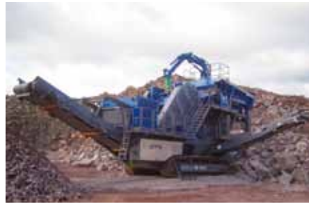
Ideally suited for the initial crushing stage: The MC 125 processes lumps of rock up to a feed size of 48" x 36" (1,200 x 900 mm).
