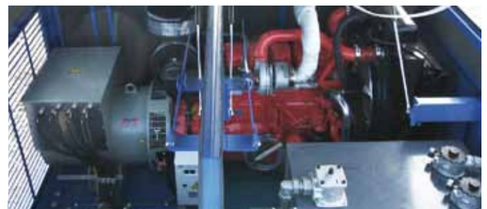
Ideally suited for the quarry requirements: diesel-electric drive concept.
