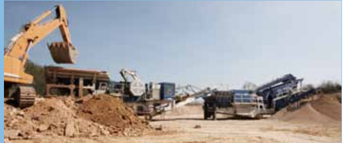
The MCO 9 S is loaded directly from a mobile Kleemann jaw crusher, MOBICAT MC 120 Z model.
