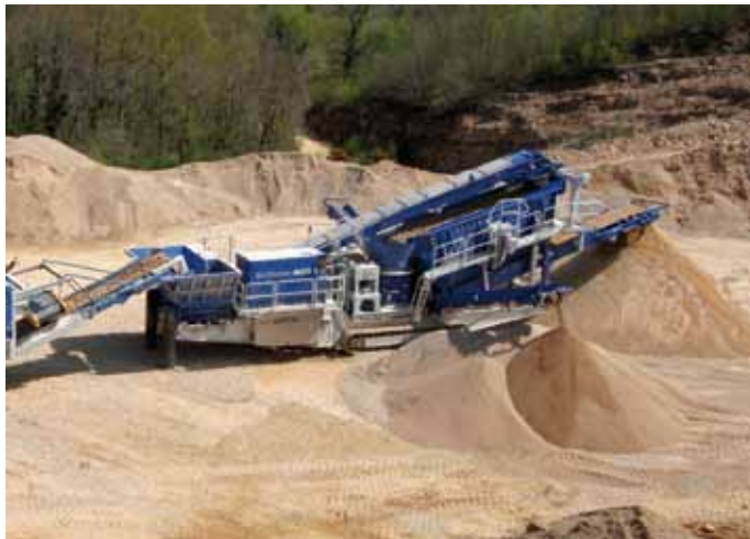
The MCO 9 S produces three high-quality product sizes in closed loop operation.
