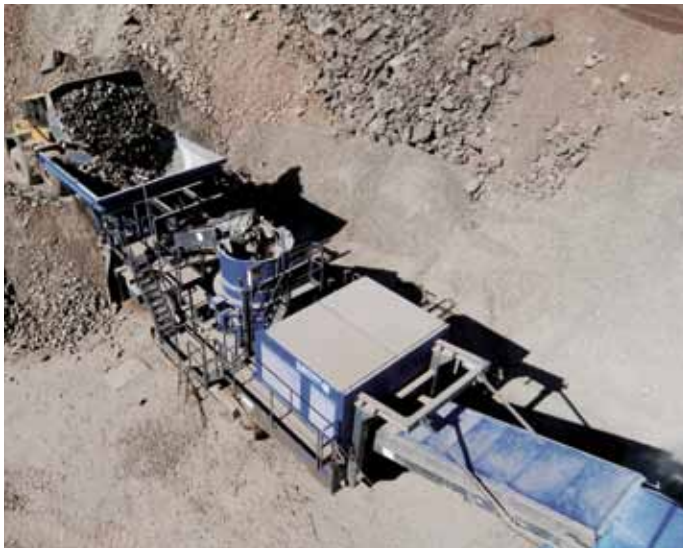
The MCO 11 can also be loaded using a wheel loader.
