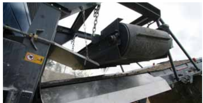
The powerful electromagnet (optional) reliably sorts the reinforced steel.
