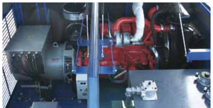
Ideally suited for quarries: diesel-electric drive concept.
