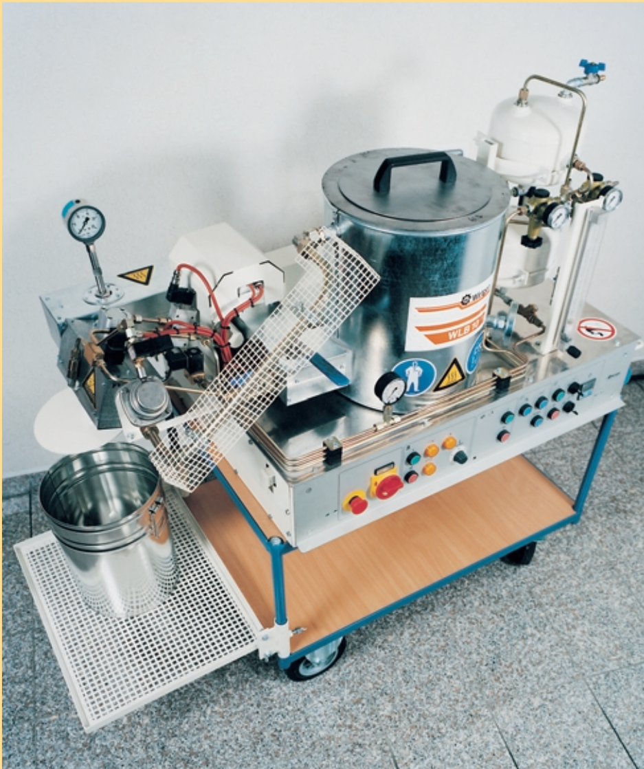
Practical: the laboratory-scale foamed bitumen plant WLB 10 on a mobile table. The tank for the foamed bitumen is on the left.
