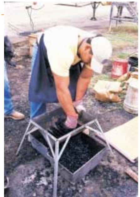
Frontera Materials technician checks Superpave sample
