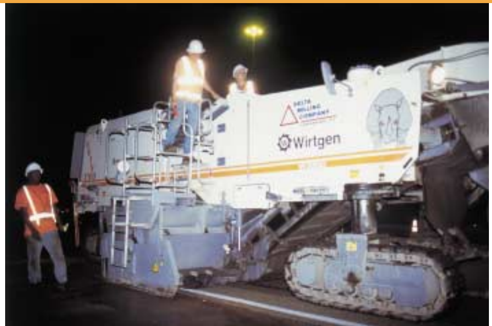
W 2200's 12-foot drum mills in one pass
