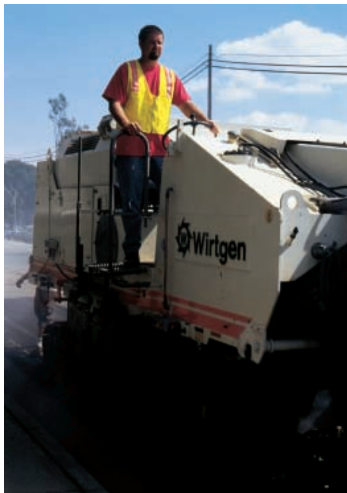
Operator Bobby Moody uses 1900 DC to mill in Ontario, Calif
